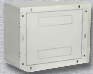
Cable entries are prepared in the top and bottom of the cabinet, two of them are also located at the back side of the cabinet. Each cable entry is blanked with a "break-out" style blanking panel that can be easily broken out by a simple tool like a screwdriver.
